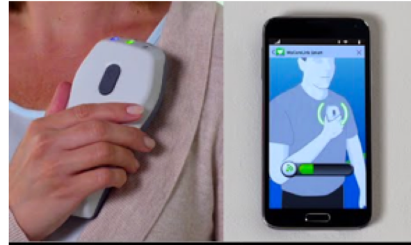
Medtronic MyCareLink Smart™ The reader (left) interrogates the ICD and sends medical data to smartphone app via Bluetooth
